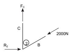
During analysis of node 1,  $F_B$  was found to be 2000N and was not negative so the assumed direction towards the node (compression) was correct.
