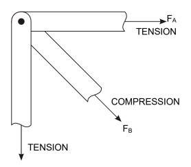
$F_{\tt B}$  is under compression and pushes into the node,  $F_{\tt A}$  is under tension and pulls away from the node.
