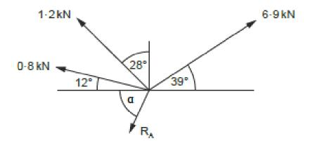
Calculate the magnitude of the reaction force  $R_{\text{A}}$  and the angle  $\alpha$
