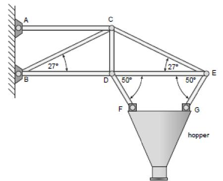
For a particular load, members DF and EG are each subjected to a tensile force of 78 kN.
