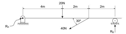
**Note:** The reaction at a roller support is always at right angles to the surface. The direction of  $R_A$  is assumed. If any of the components work out as negative values then the direction will be opposite the assumed direction.
