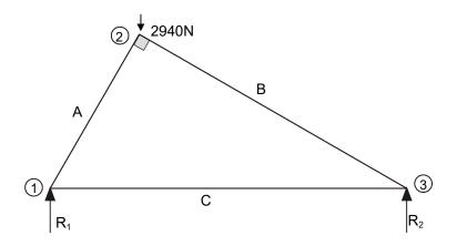
In this type of problem where the structure is acting as a beam, find R1 and  $\mathsf{R}_2$  using moments.
