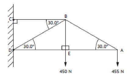
(c) Calculate, using nodal analysis at nodes A and B, the magnitude and nature of the forces in members AB, AE, BD, and BC.
