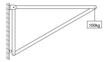
Draw a free body diagram of the frame structure.
