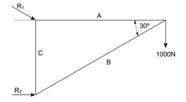
If a wrong assumption about the member being in tension or compression or the direction of a force is made then a negative value will be produced from the calculation. If this is the case the direction of the force is simply reversed
