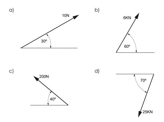
2. Find the resultant for these force systems. Find the horizontal and vertical components of each - add them up to find the overall component forces and then find the resultant.
