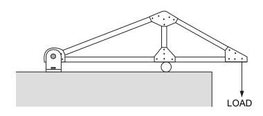
The load acting on the frame structure above will have a turning effect on the structure.
