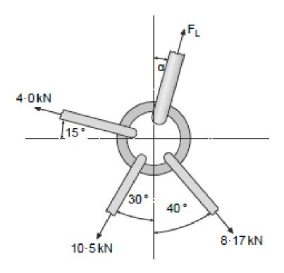
For the forces shown, calculate the magnitude and direction of force  ${\rm F_L}$  in the link.
