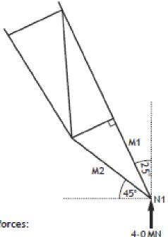
Step 1 - Establish an equation for the sum of the horizontal forces:
