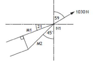
Calculate, using simultaneous equations, the magnitude of the forces in members M1 and M2.
