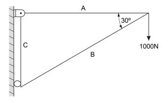
The framework is supported at two points. The hinge support at the top is being pulled away from the wall.  $R_1$  will act against this pull and keep the hinge attached to the wall. The roller support is being pushed into the wall.  $R_2$  will act against this force and in the opposite direction as shown below.
