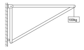
The members in this framed structure can be as ties or struts, depending on the type of force they support.
