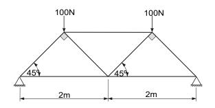
Treat structure like this as a beam and use moments to find reactions. Until the reaction forces are found all nodes have more than one unknown force or component.
