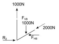
$F_{c}$  will be equal and opposite to the Vertical component of  $F_{B}$  ( $F_{VB}$ ).
