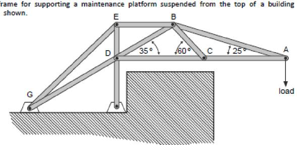
A frame for supporting a maintenance platform suspended from the top of a building is
