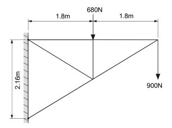
As all vertical forces acting on the node must equal zero then  $\mathsf{F}_V$  must equal 900N.
