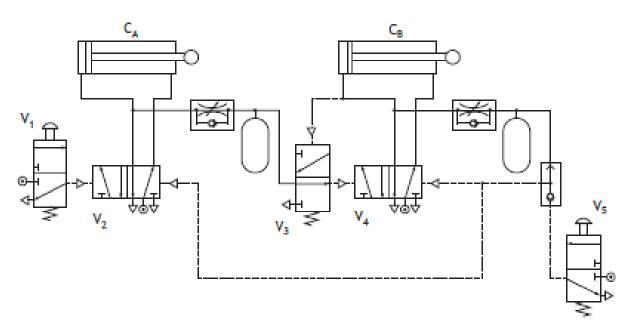
(c) Describe, with reference to the components, the full operation of the pneumatic circuit when the button on V<sub>1</sub> is pressed.
