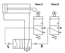
As the piston instrokes, it trips valve A and the 5/2 valve changes state and the piston is sent positive. When it is fully outstroked, it trips valve B and the 5/2 valve returns to its original position, allowing the piston to instroke. The process begins all over again and continues to operate.
