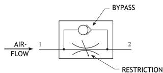
When air flows into port 2 of the restrictor, again some of the air takes the bypass route. This time, the ball is blown away from the valve and the air passes through unrestricted.
