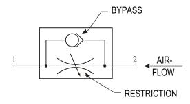
In pneumatics, unidirectional restrictors are much more useful to us. However, we must always be careful to insert them in the circuit the correct way round.
