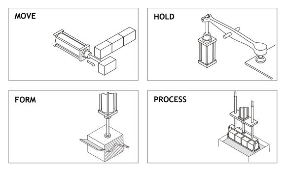
Every one of these pneumatic systems makes use of *compressed air*. Compressed air is quite simply the air that we breathe forced or squashed into a smaller space. We can use the energy stored in this compressed air to do things.
