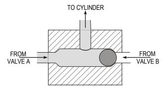
When air is supplied from valve A, the ball gets blown across and the air is directed towards the cylinder. When air is supplied from valve B, the ball is blown to the other side and again the air flows into the cylinder. If air comes from both directions, air still manages to reach the cylinder, as this is the only path it can take.
