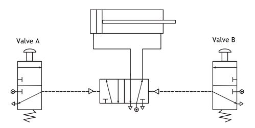
Notice that the pilot airlines to the 5/2 valve are drawn as broken or dashed lines to distinguish them from the other air lines in the circuit.
