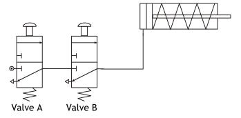
The single-acting cylinder will only outstroke when valve A *and* valve B are pressed at the same time. When the button on valve A is pressed, main air passes through and reaches valve B. The air cannot flow any further until valve B is pressed. This then supplies the cylinder with air and it outstrokes.
