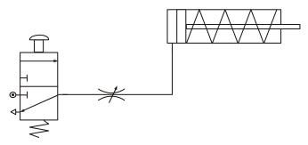
The problem with this type of restrictor is that it always slows down the speed of the piston in both directions. In many cases, we would only want either the outstroke or the instroke to be slowed down. Also, if we study the piston movement very carefully, we sometimes find that it is quite jerky and not smooth as we would want it to be.
