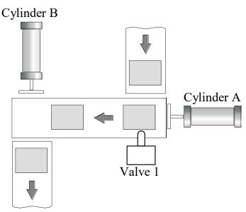
The sequence of operation of the cylinders is A+, B+, A-, B-.
