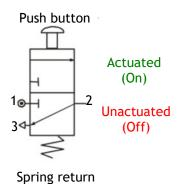
The **states** in the valve are simply **actuated** (on) or **unactuated** (off). The symbol for the valve shows how the valve is operating when in either of its two states:
