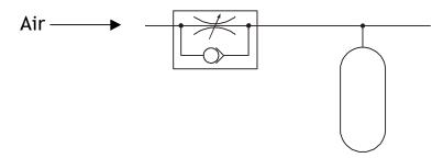
We can change the length of a delay by changing the size of the reservoir or adjusting the restrictor.
