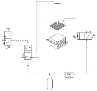
When the push button is pressed, the 5/2 valve changes state and the cylinder outstrokes. As it outstrokes, it pushes the former together and the hot plastic sheet is pressed into shape. As this happens it also actuates the roller. Air now flows through the restrictor and starts to fill up the reservoir. Once the reservoir is full, the 5/2 valve changes state and the cylinder instrokes, ready for the process to begin again.
