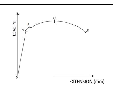
'A' - Limit of Elasticity and any loading beyond this point results in plastic deformation of the sample.
