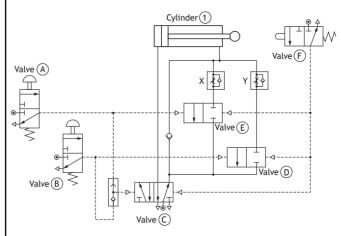
(a) Describe, with reference to all of the components in the pneumatic circuit, the operation of the system when valve  $\ensuremath{\mbox{\/ A}}$  is pressed and released then valve (B) is pressed and released.
