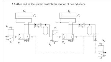
Describe, with reference to the components, the full operation of the pneumatic circuit when the button on  $V_1$  is pressed.
