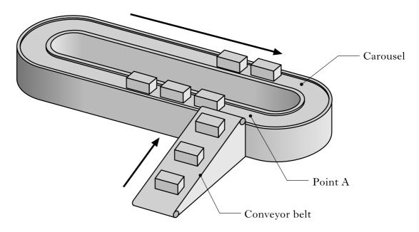
Bags are added to the carousel by a conveyor belt. If bags are detected at point A, the conveyor belt will automatically halt until there is space on the carousel for more bags.
