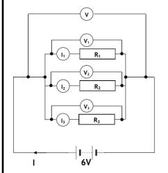
$V = V_1 = V_2 = V_3$  (Voltage stays the same)
