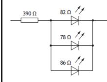
Calculate the resistance of the 3 LEDs in parallel.
