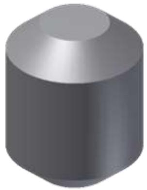
Completed Revolve with Chamfer
